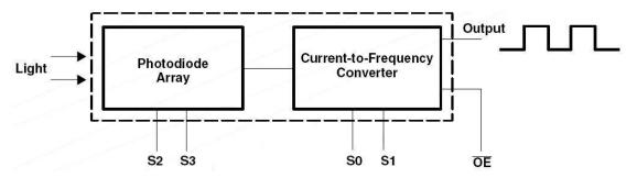
TCS3200D contains four types of filters: red filter, green filter, blue filter and clear with no filter. When the sensor is illuminated by a ray of light, the types of filters (blue, green, red, or clear) used by the device can be selected by two logic inputs, S2 and S3. Table 2 illustrates the relationship among S2, S3 and filter type.
